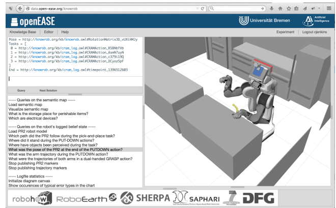
Fig. 5. The openEASE project by Tenorth, Beetz, et al. is an example of robot operation and semantic mapping through RWT.
